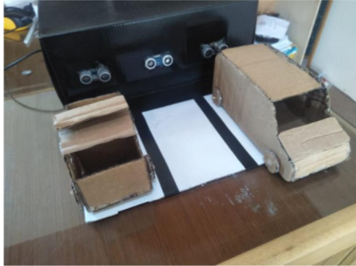
Fig. 4 Implementation of a Car Parking Distance Controller
