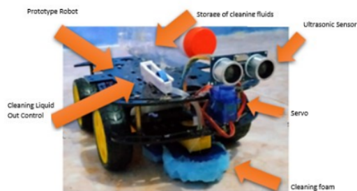
Fig. 6. Automatic Floor Cleaning Robot Prototype detects distance
