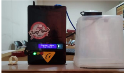
Fig.9. Implementation of Smoke Detection and Neutralization Tools
