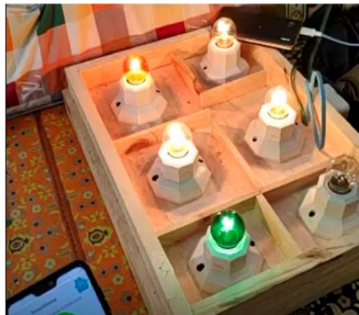
Figure 3. Implementation Results of prototype house lights controlled from Android
