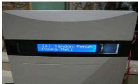
Fig. 4. the pump shuts down automatically
